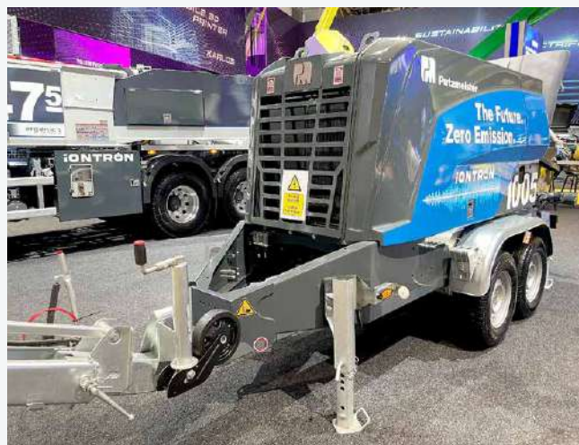
> Putzmeister concrete pump
